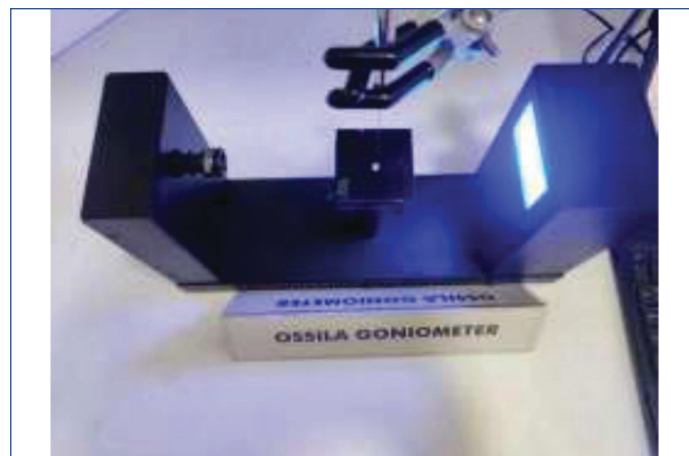
[Table/Fig-3]: Ossila Goniometer for measuring contact angle.
